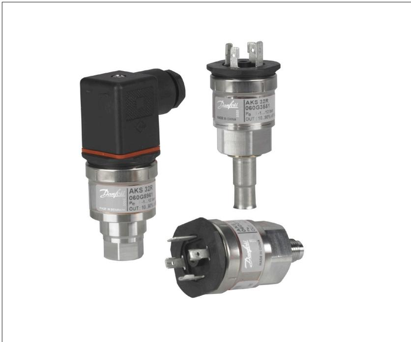
AKS 32R is a ratiometric pressure transmitter that converts the measured pressure to a linear output signal. The output signal is relative to the supply voltage meaning that the min. pressure output will be 10% of the actual supply voltage and the max. pressure output will be 90% of the actual supply voltage.
